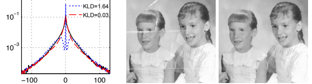
Figure 7. (Left) Derivative statistics of 10 denoised test images (blue, dotted – MAP; red, dashed – MMSE) and of corresponding clean originals (black, solid), \sigma=10, 20 . (Right) Sampling-based inpainting result (MMSE) from our learned pairwise MRF.
